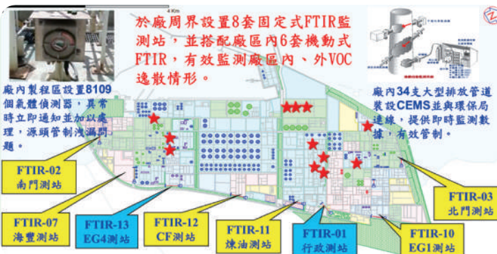
Locations of monitoring equipment inside the premises
