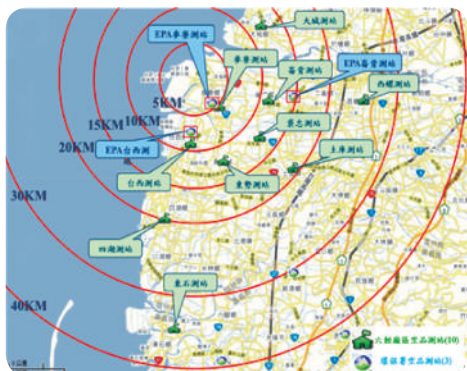
Air quality monitoring stations of the sixth naphtha cracker and EPA air quality monitoring stations
